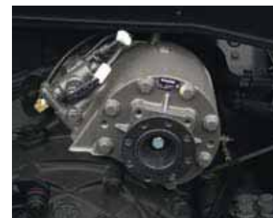
The efficient and powerful engine PTO produces power up to 150 kW.
